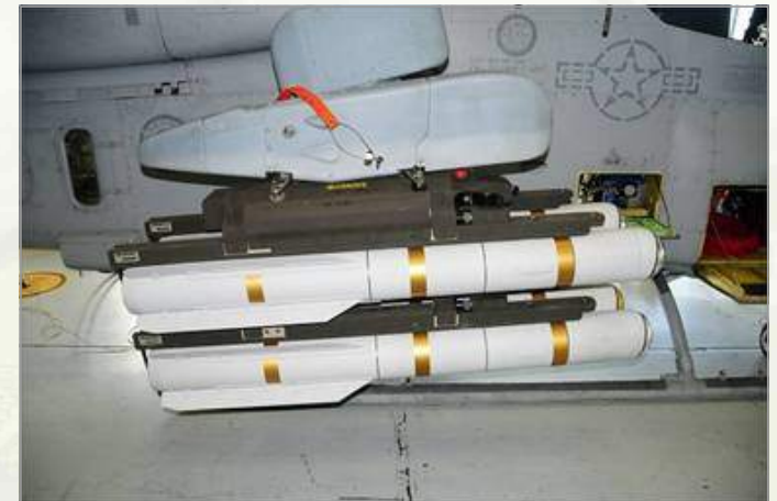
▶ Joint Air-to-Ground Missile
