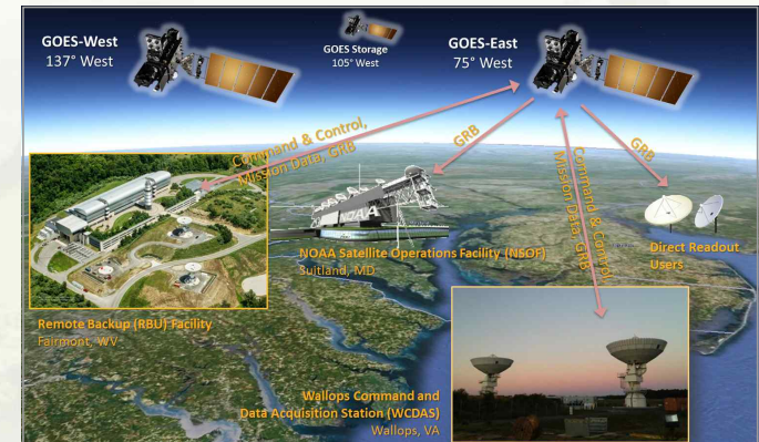
▶ GOES-R Ground Segment Architecture
