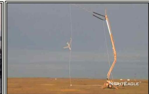
[ 출처 ] Drone on a wire: Marines land new RQ-21 UAV by snagging it with cable, 2012.8.1, defense.aol.com [ 목차로 이동 ]
